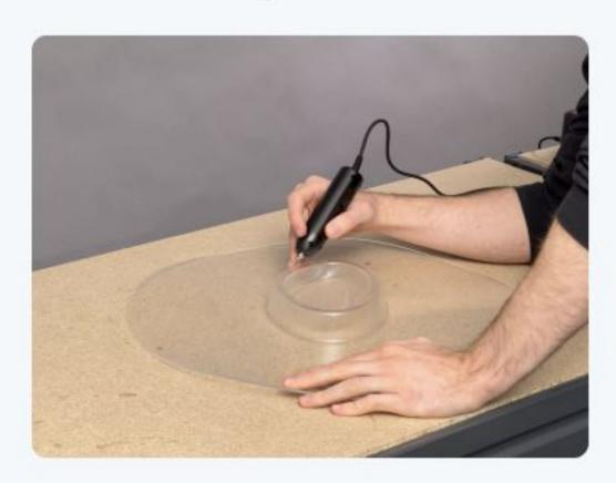
High frequency knife Use a jig for accuracy and speed
